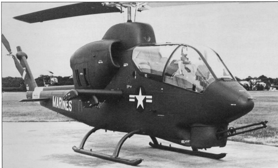
This Sea Cobra is the first of 49 readied for delivery to the Marine Corps by Bell Helicopter in Texas in 1969. It featured a three-barrel, turret-mounted 20mm cannon capable of firing 750 rounds per minute and could cruise at 185 mph and dive at 219 mph.
